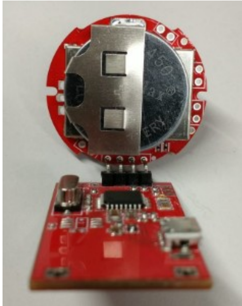
Figure 1: MReX-PROG connected to MReX-MB1
